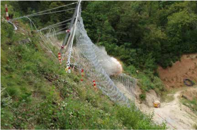
Figure 1. Flexible “hybrid” type rockfall barrier during testing. (Photo courtesy of Tom Badger, Golder Associates, Inc.)
