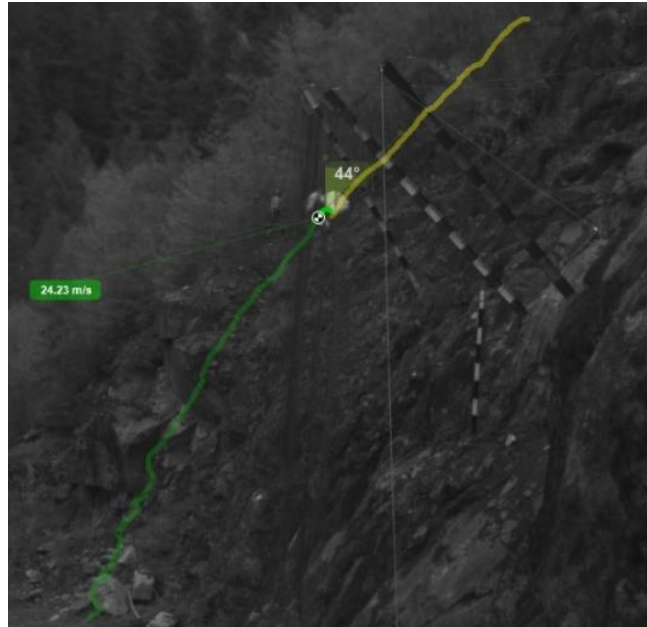
FIGURE 10 Tracking of a block throughout its fall with the software Kinovea.
