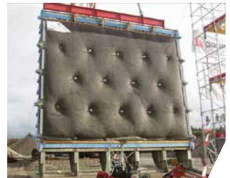
Fig. 32: Test no. 5, TECCO® G65/3 + P33, = 85^\circ , sandy gravel 0 - 63 mm
