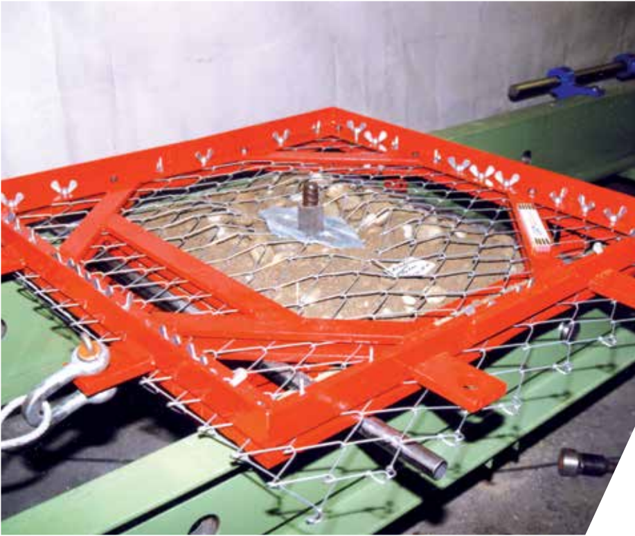
Fig. 27: Test setup to determine the bearing resistance of the mesh against selective tensile stress parallel to the slope
