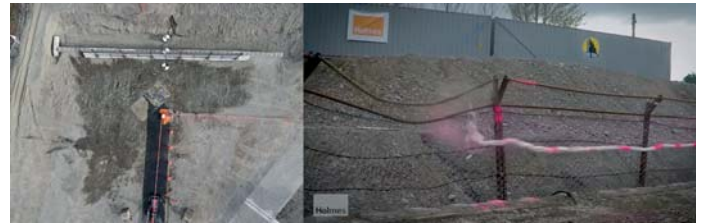
Full-scale test setup and validation of Geobrugg's Snapback Protection Systems
