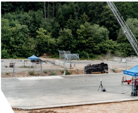
Barrier is tested with 9 elements (36 meters), not as a "single field barrier". Minimum length: 20 meters.
