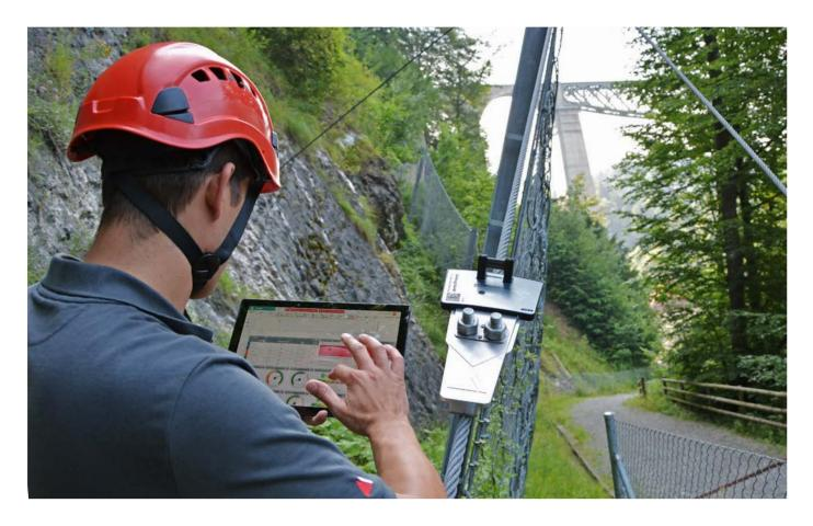
The Geobrugg GUARD lives up to its name: This smart device monitors your protective structures by providing the most important information. With an installation time of under five minutes, online monitoring becomes almost instant, ensuring the condition of your protective structures is always only one click away.
