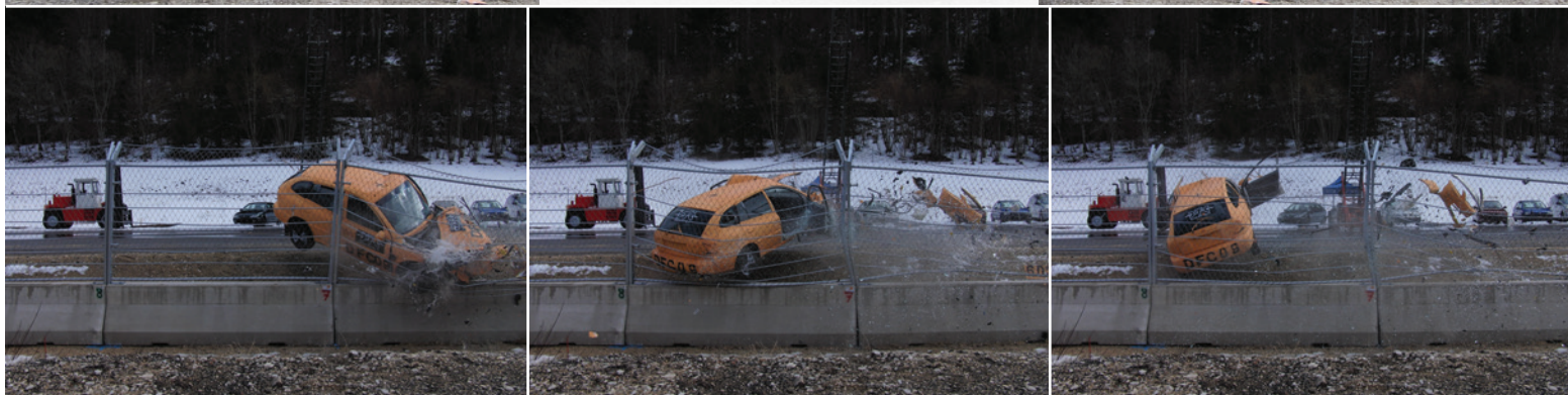
ABOVE & BELOW Testing times: bespoke tests were devised, including a steel sphere (above) and 1,000 kg car (below) being fired at the debris fence at specific angles
