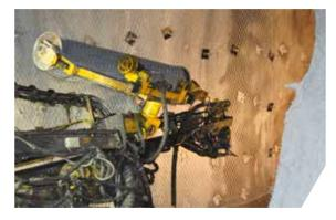
Above: MESHA® can be retrofitted to any multi-boom bolter.
