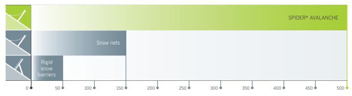
Energy absorption capacity [kJ] ▶
