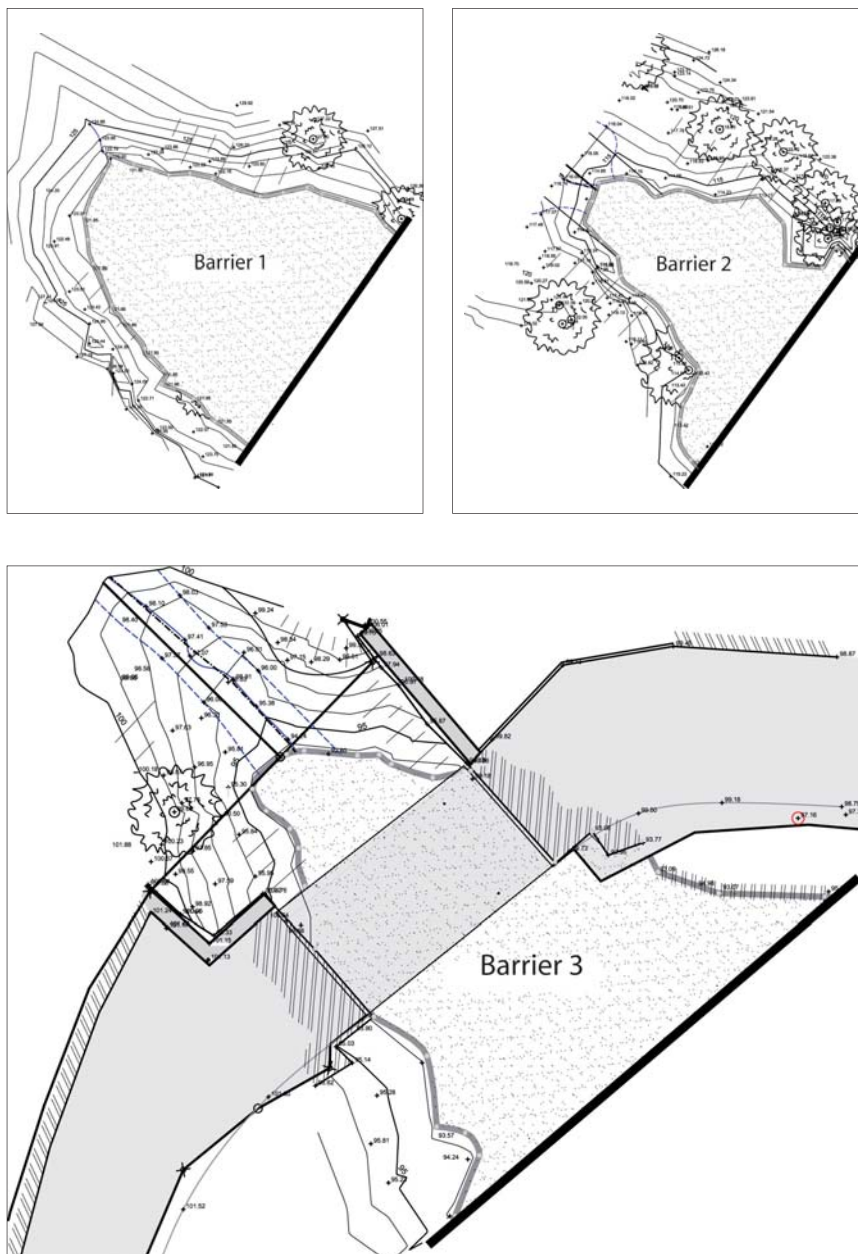
Fig. 5: Accumulation planimetry and the expected volumes of debris retained by the three barriers
