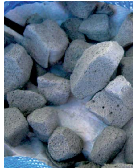
The ROCKFALL-X™ cylinder modules are filled up with cellular glass as cushioning material
